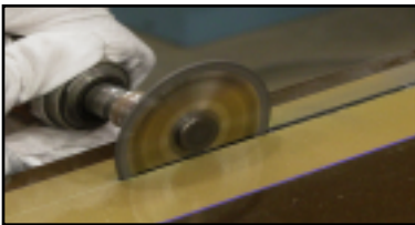
The tape is removed and marking used as a guide to trim the edge of the part
